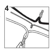
5. Attach wire nuts(D). Tape wire nuts(D) and wires together with electrical tape.
