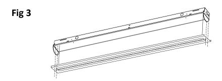
**Step 6** . A. If mounting to the 4 inch JBox, assemble the cover plates into fixture.
