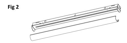
Step 5 . Take off LED module plate from the body of fixture. (Caution: avoid to touching LEDs)
