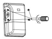
4. Screw the bottom plate on the wall
