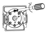
7. Fix the fixture by 4 screws
