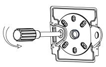
7. Return on the fixture to the bottom plate and tighten it with screws
